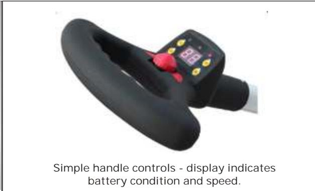
Simple handle controls - display indicates battery condition and speed.
