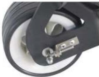
Front wheel tracking adjustment both sides
